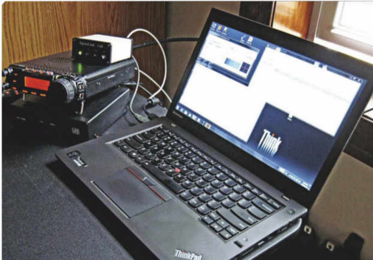
◀ Left: Radio on and software running, stations can be left unattended and connected to peer-to-peer (P2P) to exchange email messages. This frees the operator to do other tasks and not worry about missing important communications.
