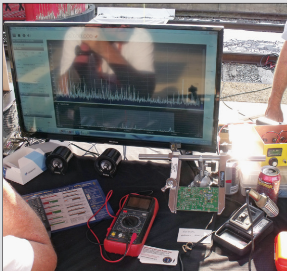
The spectrum display in the back came from a 2-inch x 3-inch SDR receiver connected to a vertical on a tripod. In the foreground are ham "Maker" tools; a meter, a PanaVise®, and a soldering iron.
