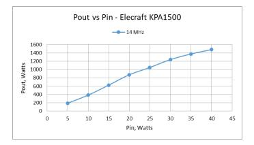
You can eyeball a straight line on this plot, and you'll conclude that the Pout vs Pin data does deviate from the straight line. But what does that mean?
