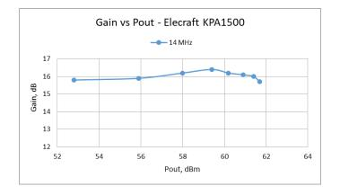
To answer this question, a better way to characterize a PA is to use the same data from the Pout vs Pin plot, but plot Gain in dB vs Pout in dBm. Here's that plot for the KPA1500 on 14 MHz:
