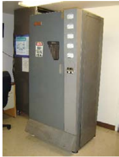
GATES BC-1T AM BC TRANSMITTER 1 KW (2) 807 DRIVING (2) 833A, MODULATED BY (2) 833a ORIGINALLY USED AT KPGE, PAGE ARIZONA, 1340 KHZ
