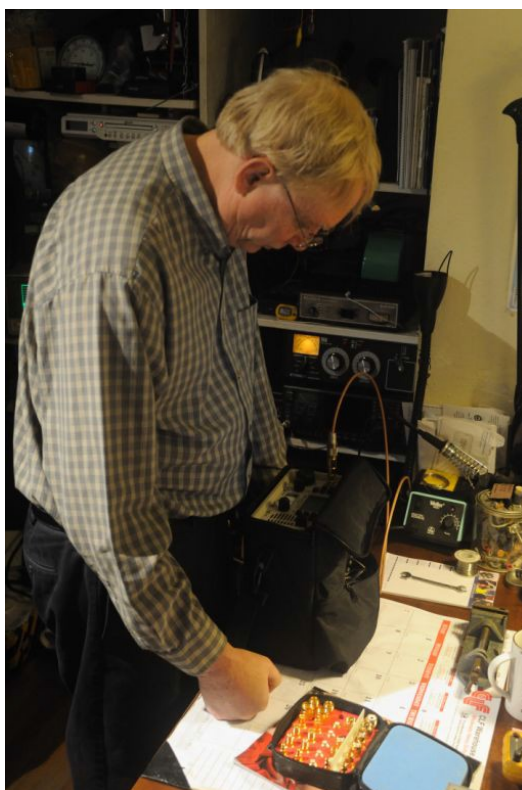
Figure 4 - Observing the noise as it affects a complainant's station is a critical step in the process. In this photo, the RFI Investigator is connecting his locating receiver to observe and record the noise that is the source of this complaint.
