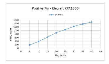
You can eyeball a straight line on this plot, and you'll conclude that the Pout vs Pin data does deviate from the straight line. But what does that mean?
