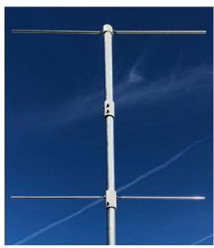
**LinkedIn:** Bolster your operation for long-term use anywhere with "A Compact 2-Meter Base Station Antenna for Rugged Use" by John Portune, W6NBC. Made from thick-wall aluminum and under 25 inches in height, this antenna will withstand mountaintop winds for years. Read about it in the September 2019 issue of #QST, online now or in your print edition arriving soon.
