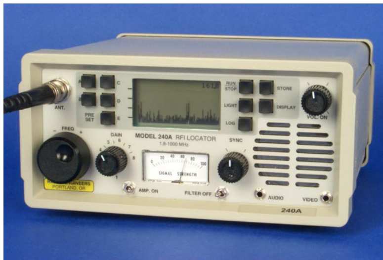
Figure 3 - The Radar Engineers Model 240 HF-UHF RFI Locator is a professional grade receiver for locating RFI sources. It has a built-in oscilloscope display for recording and observing noise signatures. This receiver operates from 1.8 to 1000 MHz.
