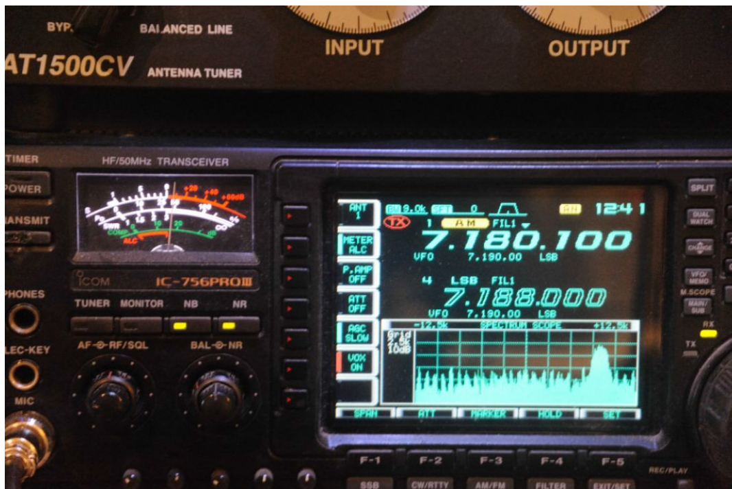
Figure 2 - The noise as it affected Mr. Schreiber's station during the initial phase of our investigation. It registered well over S9 on the S Meter.
