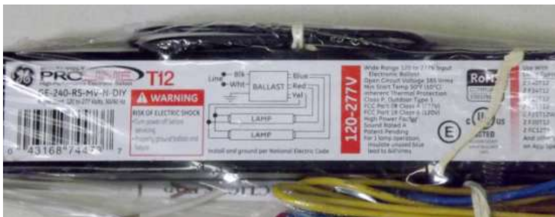
Figure 3 – Close-up of T12 ballasts in the center box shown in Figure 2. As can be seen in this photo, this ballast is labeled FCC Part 18 “Class A” (277V) and FCC Part 18 “Class B” (120V). It can be either a consumer or non-consumer device, depending on the voltage.
