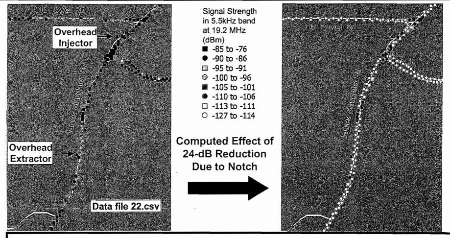
Highest emission from BPL is reduced to -100 dBm, 4-dB lower than the maximum seen in driving past the substation and 14 to 27 dB above ambient.
