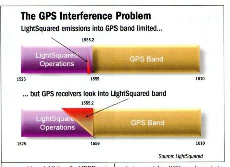
not tracking. Additionally, NPEF tests showed that even lower-band transmissions would interfere with high-precision GPS receivers used in construction and agriculture.
